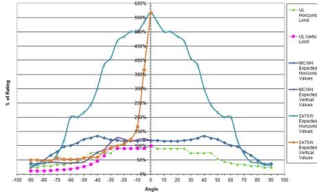
Figure 5: Expected light output for Ceiling (left) and Wall (right) Models
