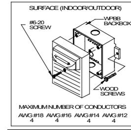
**WARNING:** This unit must be mounted on a flat surface, so that the surface covers the entire back surface of the backbox. When used in an outdoor application or a NEMA 3R application, use weatherproof-rated conduit fitting on all knockouts of the backbox.
