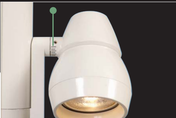
Lampholder arm employs graduations every 15^\circ for precise, repeatable tilt aiming. An indicator mark on arm bottom assures perfect lamp housing alignment with the track.
