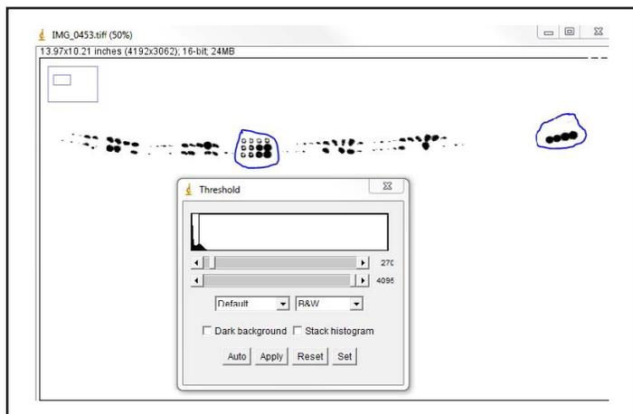
**Figure 3. Areas exceeding threshold of 1500 Candela/M2 (LED fixtures circled in blue)**
