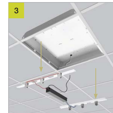
Remove Ballast / Sockets
