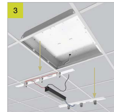
Remove Ballast / Sockets
