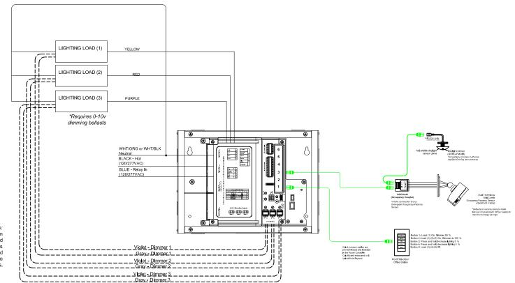
\*0-10V Dimming Zone Note: The 0-10V dimming zones within the Room Controller can be wired and controlled independent of the connected loads. This allows a each load to have a dedicated 0-10V dimming zone or a single load to have up to three 0-10V dimming zones.
