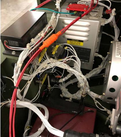
**Figure 4.** In-line fuse holder application
