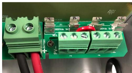
Figure 3. 600 Vdc PCBA with fuse clips
