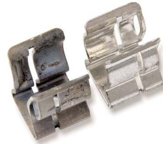
The fuse clip on the right has excellent tension that provides a good mechanical and electrical interface (low resistance) between the fuse and clip. The clip on the left experienced excessive thermal conditions due to an improper conductor termination or undersized conductor. As a result, the clip lost its tension. Consequently, the mechanical and electrical interface between the fuse and clip was not adequate which further accelerated the unfavorable thermal condition.
