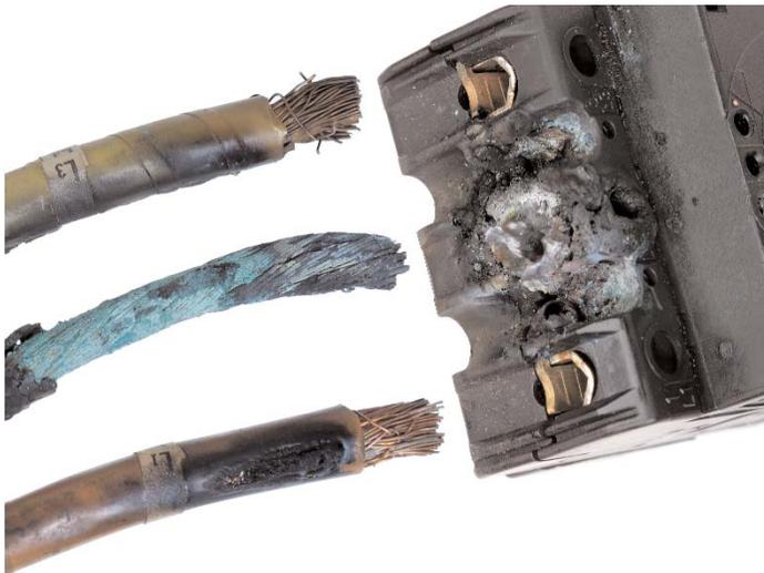
The middle, line-side conductor to this disconnect became loose. The loose connection created an excessive thermal condition that caused excessive damage to the device termination, the middle conductor and the adjacent conductors.
