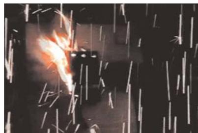
Photo (later in sequence) of 3-pole circuit breaker during test of individual single-pole interruption of a fault current beyond its single-pole interrupting capability - it violently exploded.
