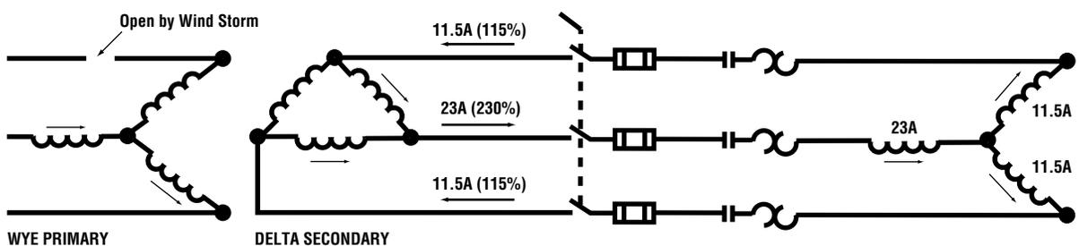
Figure 5B. (Wye-Connected Motor) Diagram showing how the phase currents to a three-phase motor increase when a single-phasing occurs on the primary. For older installations where the motor is protected by two overload devices, the phase winding having the 230% current will burn up. However, properly sized overload relays or LOW-PEAK® or FUSETRON® dual-element, time-deady fuses will clear the motor from the power supply.
