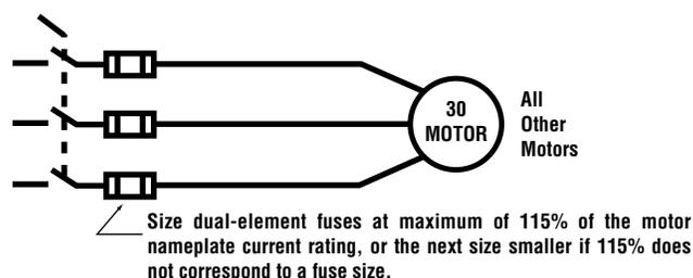
Figure 6B. All Other Motors (Over 40°C or Less Than 1.15 S.F.)
