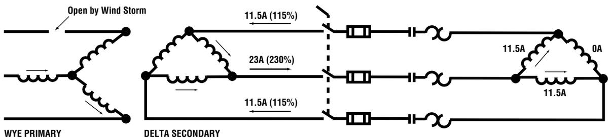
Figure 5A. (Delta-Connected Motor) Diagram showing how the phase currents to a three-phase motor increase when a single-phasing occurs on the primary. For older installations where the motor is protected by two overload devices, the phase winding having the 230% current will burn up. However, properly sized overload relays or LOW-PEAK® or FUSETRON® dual-element, time-deady fuses will clear the motor from the power supply.
