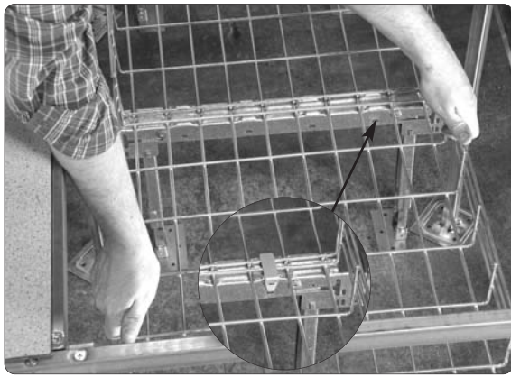
Step 1. Install first tier with baskets and clips.
