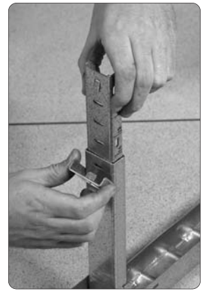
Step 2. Assemble stands with legs in outer position and adjust height.
