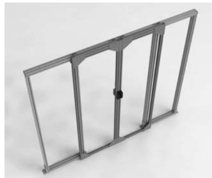
Figure 2 This view highlights the frame the door slides on.
