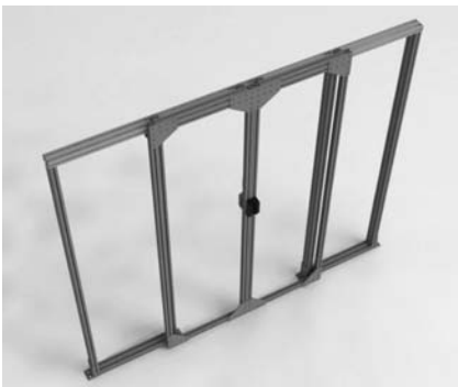
Figure 3 The view highlights the door frame header track which needs to be fixed to the door support frames before mounting to the cabinets. For assembly details see Figure 4.
